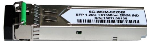
1000Base-BX WDM Singlemode (TX 1550 nm – RX 1310 nm)
